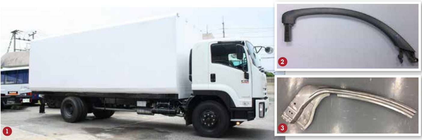
Figure 1: Light-weight Composite Container for a Six-wheel Logistic Truck reduced more 50% weight from normal (courtesy of 'GRE COMPOSITES COMPANY LIMITED')
